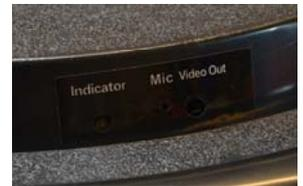
The signaling LED is very important because it makes you understand the status and this way we can know that commands impart.
