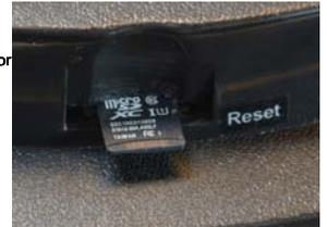
MB / s. Do not use the SD card with a lower rate because it would lead to malfunction. Attention to the direction of insertion of the SD card that will slide in its seat only with the gold contacts facing downwards, as shown in the figure. The SD card should be pushed into the slot with the nail until you feel the retaining snap. To pull it must not pull it outward, but push again until you hear the unlocking.
