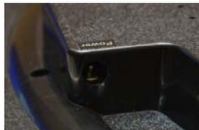
insert 220V / 5VDC supplied adapter.
